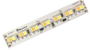
The 6949-DimToWarm strip replicates a halogen lights warming effect. Change from 4000K to 2700K by simply dimming the light with a traditional wall switch. Bring out the true color of your spaces with CRI 90+ LED chips. Deliver all the versatility of LED Strip with the same quality light as traditional lamps.
