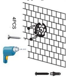
**④** Fix the lamp onto mounting bracket Tighten the 4PCS screws to fix the lamp housing onto the installation surface
