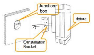
Step 2: Make connection to main wire inside the junction with insulating wiring caps(not supplied). Black wire connected to line, white wire connected to Neutral, Green wire to ground.
