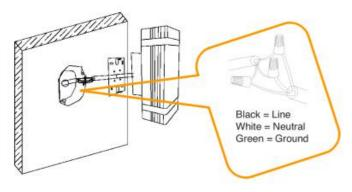
Step 3: Use screws (not supplied) to fix the installation bracket onto the junction box.
