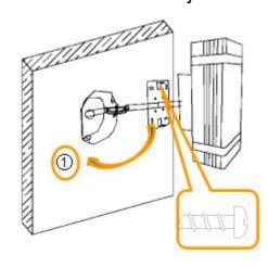
Step 4: Use (2) screws to fix the fixture on the installation bracket. After finish all the installation of fixtures, turn on the power.
