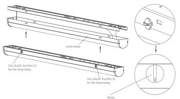
After installation is completed, the arrow must be at the vertical direction to lock the lamp body.
