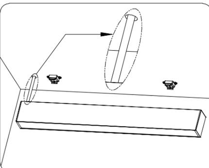
4. Thread AC input wire of lamp through another side of ceiling;
