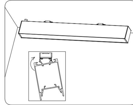
6. According above detailed figure, first snap one side on clip kits, then rotate it to install on another side of clip kits;
