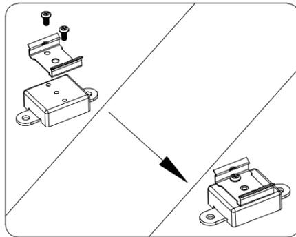
2. Fasten clip and elevated parts of clip with screws;
