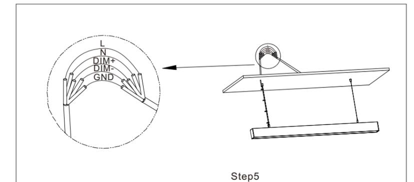
Step5: fix the fixing head 1 with fixing head 2 tightly, and adjust suspending rope with sewing machine to balance the lamp, finally connect input wire of lamp;
