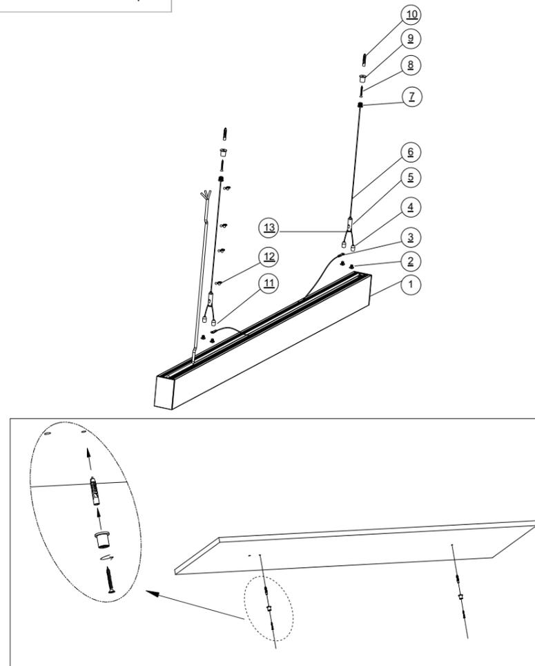
Step2: Drill hole in the ceiling, push the rubber plug into the ceiling, fix the fixing head 2 in the ceiling with 4X30PA screw.
