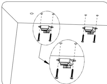
3. Fasten assembled clip kits in plastic rubber of ceiling with screws;
