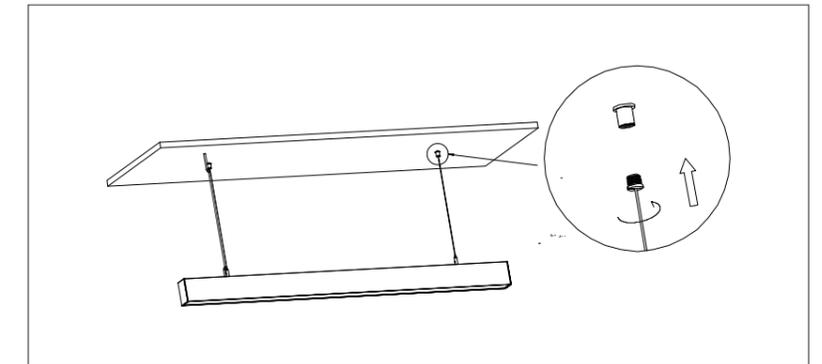
Step4: a. Suspendent method on the left: thread the power wire through 8-figure buckle fixed on the left, then install the whole set of fixing clip on the lamp;
