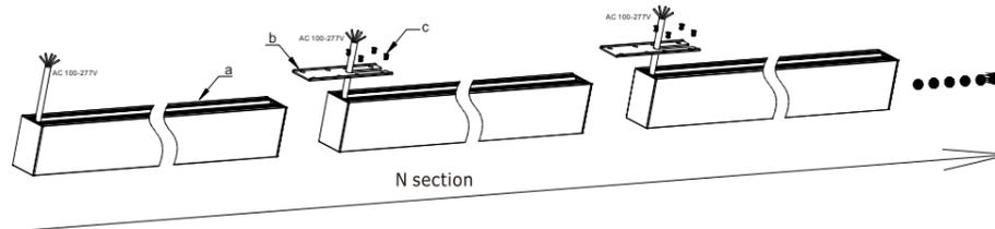
1.Snap AC input wire of lamp head into U-shape notch of connected section, then align fixing hole of connected section to fixing hole on lamp, finally fasten connected section and lamp with screws;
