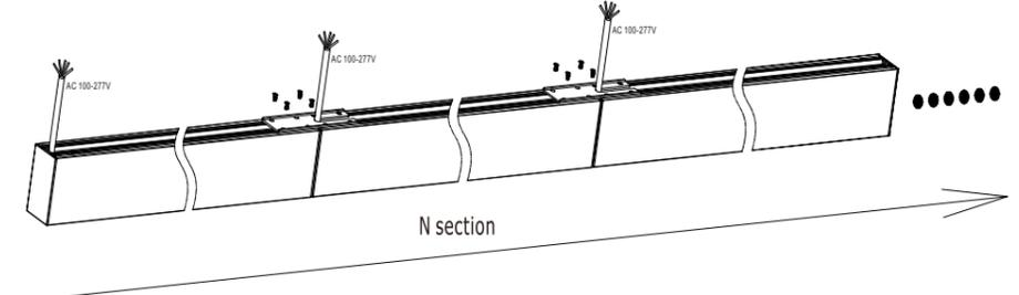
2.Align fixing hole of other side to fixing hole of lamp tail, then fasten connection section and lamp;
