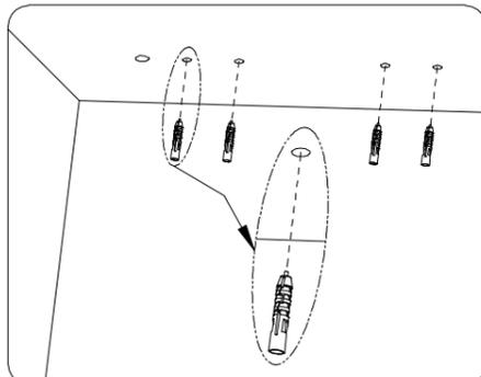
1. Plan hole distance, and drill 4 holes of 3.0mm f and 1 hole of 10.0mm f;
