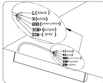
7. Connect AC according mark on the input wire, then illuminate lamp, installation finish.
