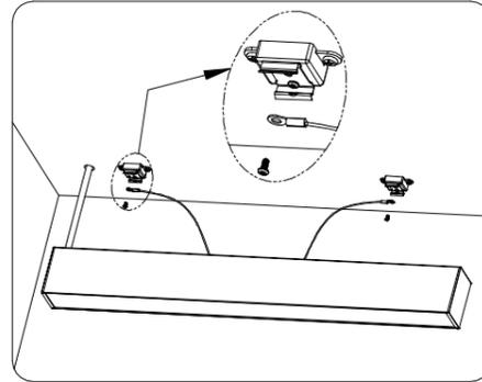
5. Thread screw through fixing hole of safety hole, then fasten it with clips kits;
