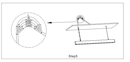
Step5:fix the fixing head 1 with fixing head 2 tightly, and adjust suspendent rope with sewing machine to balance the lamp, finally connnect input wire of lamp;
