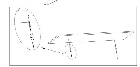
Step2:Drill hole in the ceiling, push the rubber plug into the ceiling, fix the fixing head 2 in the ceiling with 4X30PA screw.
