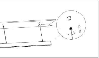
Step4:a. Suspendent method on the left: thread the power wire through 8-figure buckle fixed on the left, then intall the whole set of fixing clip on
