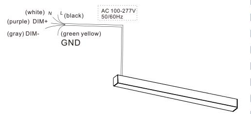
(Remark: The max current consumption of our driver to 0-10V dimmer is 2mA each one)
